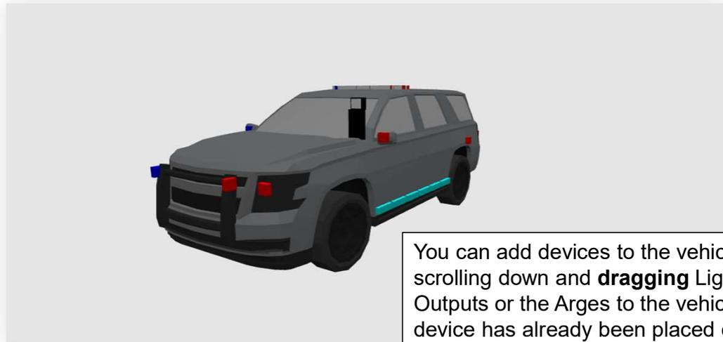
You can add devices to the vehicle model by scrolling down and **dragging** Lightbars, Outputs or the Arges to the vehicle (1). If the device has already been placed on the vehicle model it will be highlighted grey and the cursor will change from a hand to a pointer.
