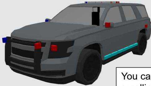
You can add devices to the vehicle model by scrolling down and **dragging** Lightbars, Outputs or the Arges to the vehicle (1). If the device has already been placed on the vehicle model it will be highlighted grey and the cursor will change from a hand to a pointer.
