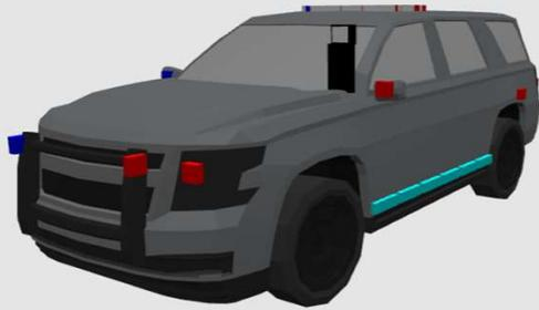
The output devices can be dragged and positioned on the vehicle. You can unlock the output devices using the **Lock/Unlock** selector (1). If at any time you move an output that you did not want to move, you can access the output menu and **Reset** the output to the snap point it was originally added to (2).
